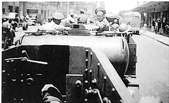
'Wasp' flamethrowers passing through Haifa, July 1946. The ignition system of the flamethrower had been dismantled and a coloured dye added to the oil. They were never used.
